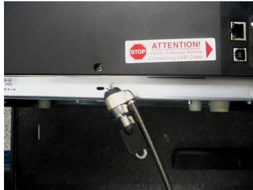
The HDPii Printer has a Security Lock Slot located in the back lip of the metal chassis to accommodate a standard laptop security lock.
