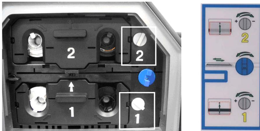
Figure 25 - Adjusting Lamination Module
